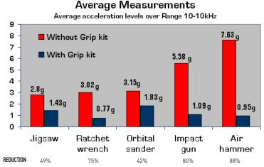
Test show average vibration reductions in a variety of hand tools after an Orthex Grip kit has been applied. Results obtained using Bruel & kjar Vibration Meter. Model 2516, for comparison only. Individual test results may vary according to hand size, grip strength, age and manufacturer of tool and other environmental factors.
