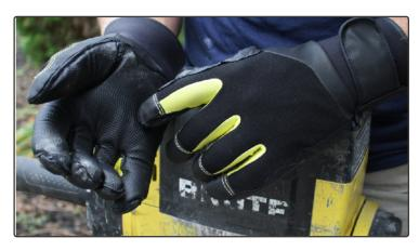
The IMPACTO AVPRO reduces vibration energy transmission to the palm, fingers and thumb. To designate a glove as Anti–Vibration per ISO 10819 standard, TR<sub>M</sub> medium frequencies must be less than < 0.90 and TR<sub>H</sub> high frequencies must be less than < 0.60.
