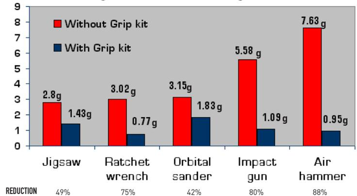
Test show average vibration reductions in a variety of hand tools after an Orthex Grip kit has been applied. Results obtained using Bruel & kjar Vibration Meter. Model 2516, for comparison only. Individual test results may vary according to hand size, grip strength, age and manufacturer of tool and other environmental factors.
